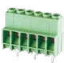
6.35mm Pitch, 600V 30A, Green, Modular Rising Clamp Standard Vertical
