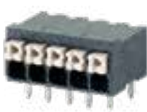
3.50mm Pitch, 300V 10A, Black, Solid Block, High Temperature Screwless Standard Horizontal
