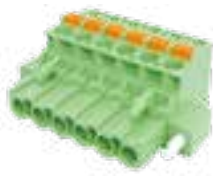
5.00mm (5.08mm) Pitch, 300V 10A, Green, Solid Block Flanged Screwless Plug
