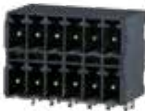
3.50mm (3.81mm) Pitch, 300V 8A, Black, Solid Block High Temperature, Double Deck Header Horizontal
