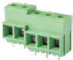
10.16mm Pitch, 300V 52A, Green, Modular Rising Clamp Standard Vertical
