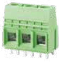
10.16mm Pitch, 600V 65A, Green, Modular Rising Clamp Standard Vertical
