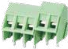
5.00mm Pitch, 300V 10A, Green, Modular Rising Clamp Standard Angled
