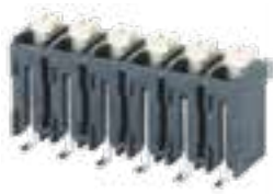
5.00mm Pitch, 300V 10A, Black, Modular, High Temperature Surface Mount, Screwless Standard Vertical
