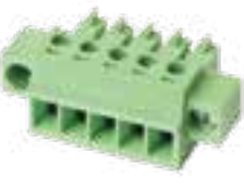
3.50mm (3.81mm) Pitch, 300V 8A, Green, Solid Block Flanged Plug With Screws
