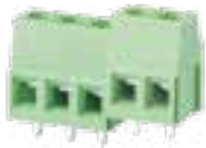
3.50mm (3.81mm) Pitch, 300V 15A, Green, Modular Rising Clamp Standard Vertical
