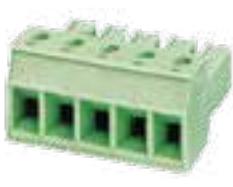
7.62mm Pitch, 300V 30A, Green, Solid Block Plug With Screws
