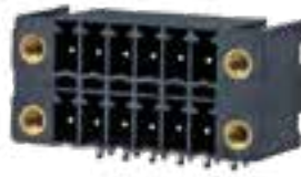
3.50mm (3.81mm) Pitch, 300V 8A, Black, Solid Block High Temperature, Flanged Double Deck Header Horizontal
