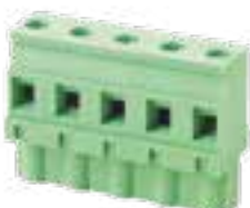
7.50mm (7.62mm) Pitch, 300V 15A, Green, Solid Block Plug With Combi Screws
