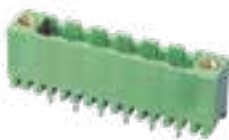
5.00mm (5.08mm) Pitch, 300V 15A, Green, Solid Block Flanged Header Vertical
