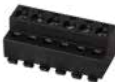
5.00mm Pitch, 300V 12A, Black, Solid Block Rising Clamp Standard Vertical
