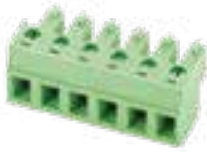
5.08mm Pitch, 300V 8A, Green, Solid Block Plug With Screws
