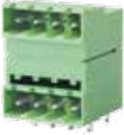
5.00mm (5.08mm) Pitch, 300V 15A, Green, Solid Block Double Deck Header Horizontal
