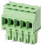
3.50mm (3.81mm) Pitch, 300V 8A, Green, Solid Block Plug With Screws
