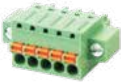
3.50mm (3.81mm) Pitch, 300V 8A, Green, Solid Block Flanged Screwless Plug
