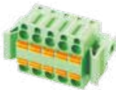
5.08mm Pitch, 300V 10A, Green, Solid Block Screwless Plug With Clip
